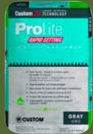
The product is capable of thin-set or medium-bed application and is formulated to allow excellent open time for adjustments while setting quickly. This permits the grouting process to begin in under three hours and enables light traffic in four hours.
